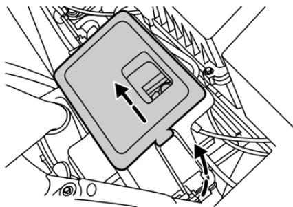
5. Remove the headlamp bulb cover by releasing the four snap hooks (two top and two bottom).
